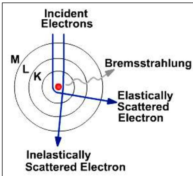
The electron may get deflected from 0-90°; if it gets a deflection of 90° (the probability of which is very small), almost all of its kinetic energy is lost and x-ray photon of high energy (equivalent to the kinetic energy of the incoming electron) will be formed. It means that an electron may lose all, none or an intermediate level of its kinetic energy in Bremsstrahlung interaction. Therefore x-ray produced will be of heterogeneous/
